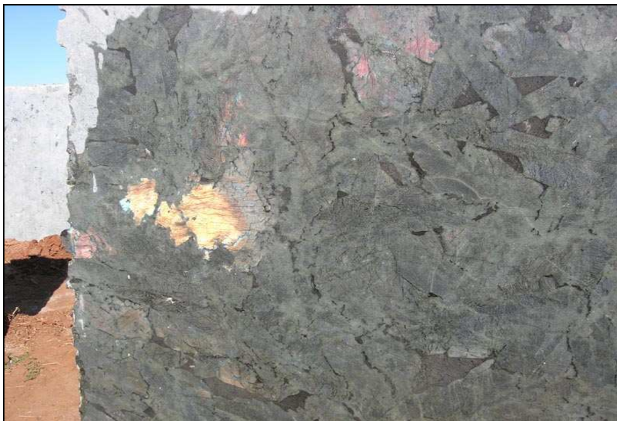
Cut face of labradorite block ready to ship, showing colour variation and crystal size. Crystals can reach the size of a small automobile
