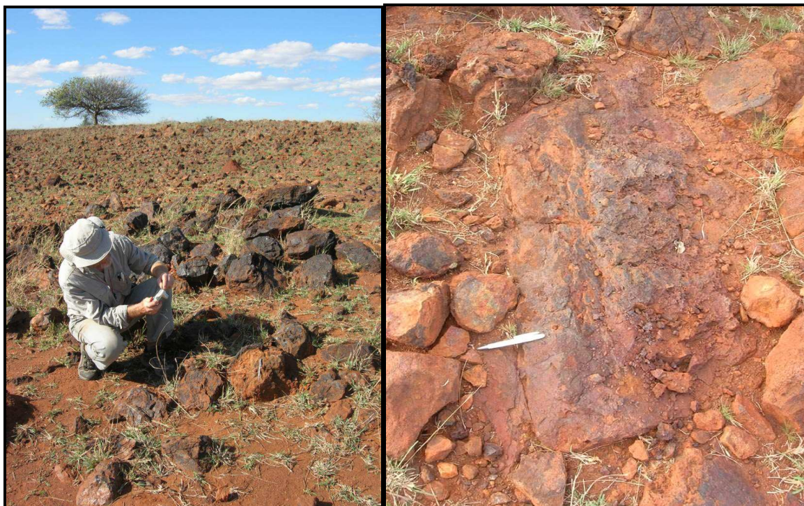
Left: Consulting nickel sulphide expert Dr. Martin Gole examining one of the Gossans at Ianapera. Right: Close-up of gossan showing characteristic texture indicative of weathered massive sulphides.
