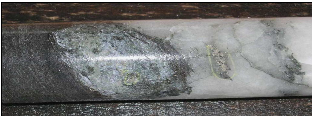
Sulphidic quartz veining in core from Vohibory Project
