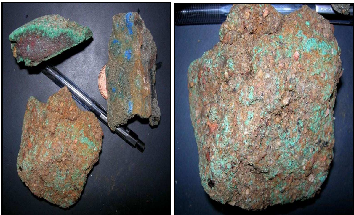
Left: Selection of typical copper-silver bearing gossans occurring in permeable units of the Isalo sediments in the VC-10 and VC-11 area. Sample in top-left of photo returned 39% Cu and 186gpt (6 ozt) Ag. Right: Close-up showing poorly sorted, immature characteristics of the sediments – note the secondary copper mineralisation permeating the interstitial areas of the rock.
