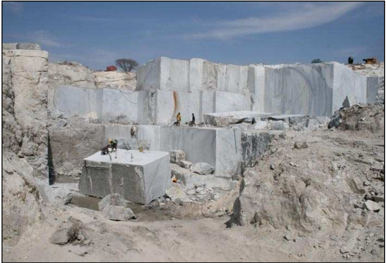
Quarrying operations in progress at one of Magrama's Ianapera quarries. Blocks are commonly quarried at around 30 tonne size and subsequently cut to 8 to 15 tonne finished blocks for road transport to Tulear.
