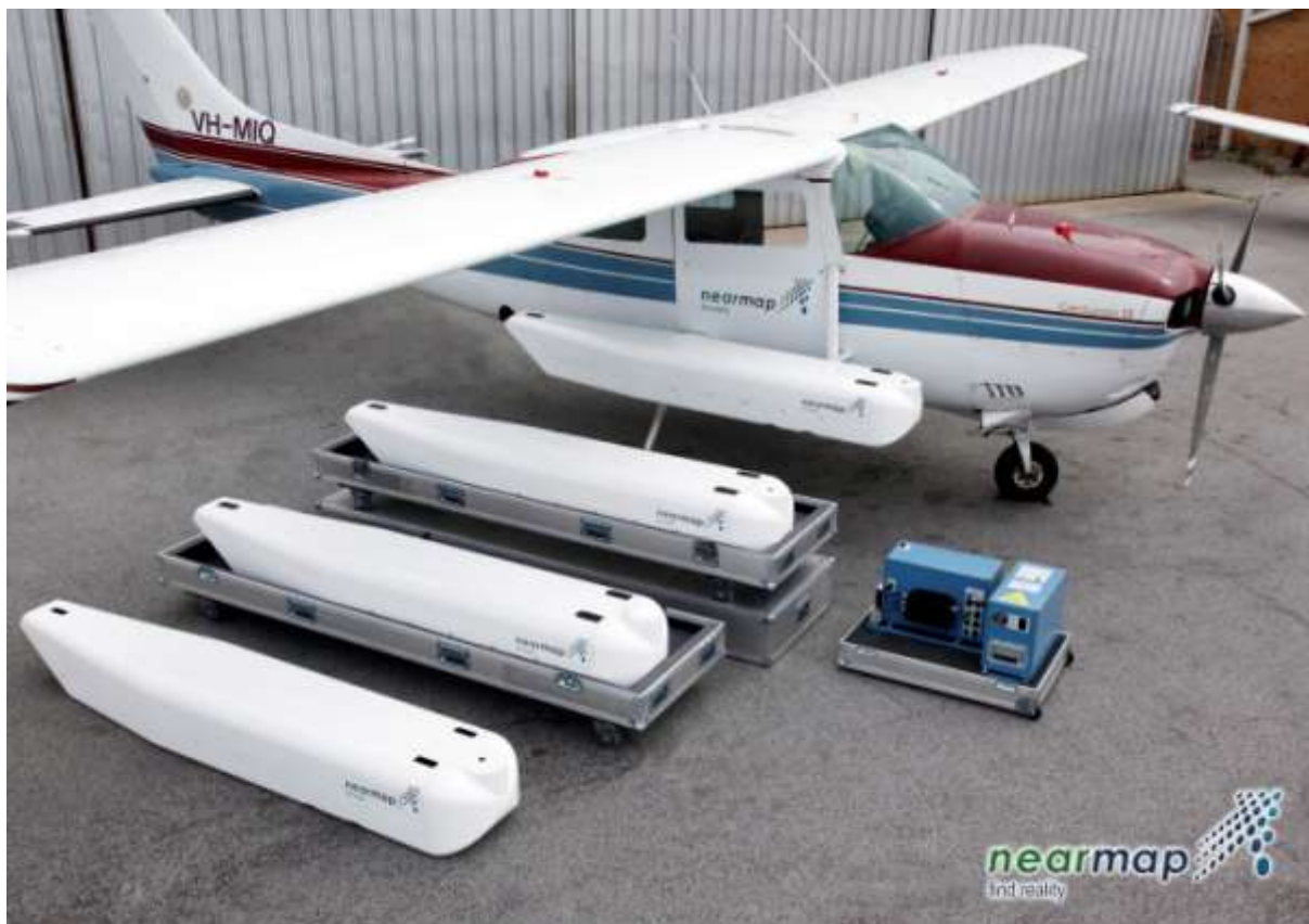
Four of NearMap's HyperPods, including one fitted to a Cessna 210 aircraft.
