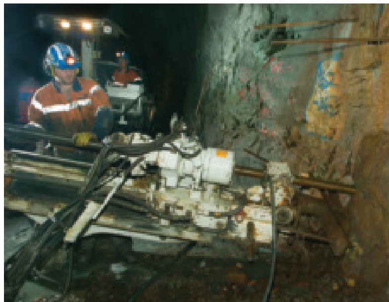
Underground diamond drilling at the Renison Mine
