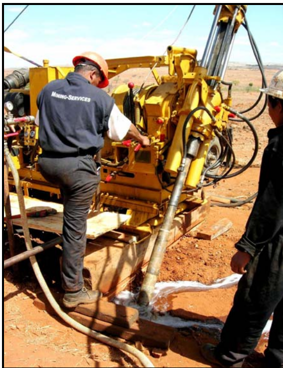
Left: Collaring the first hole (IPC0001) at lanapera Project. Right: Close-up of massive sulphides in IPC0001.
