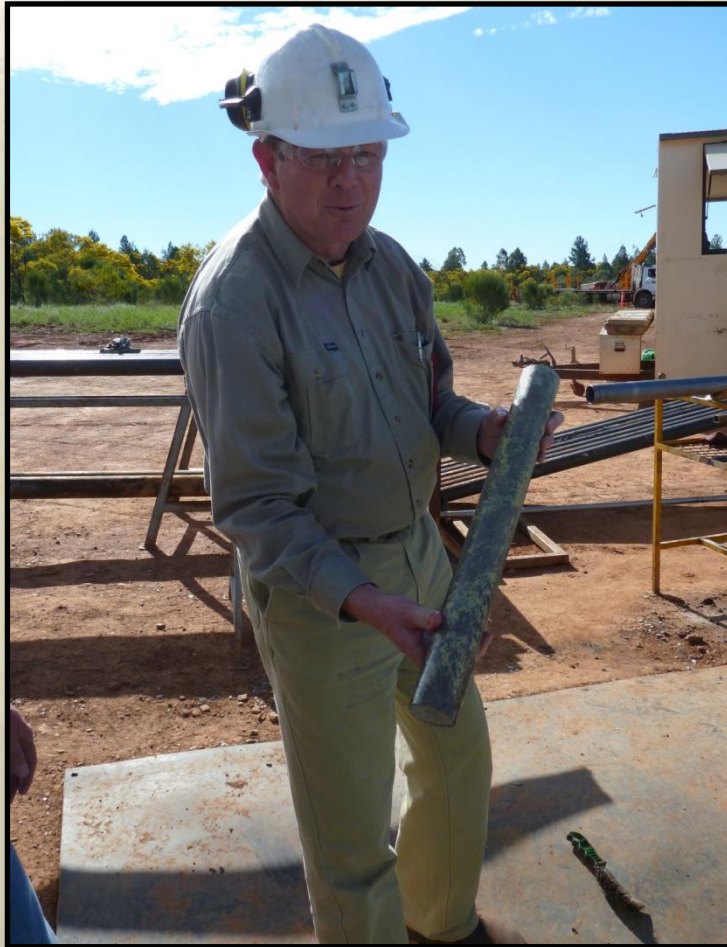
Massive sulphide core - Nymagee Copper Mine
