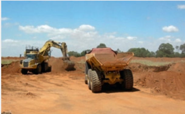
TMS Mining undertaking topsoil pre-stripping in the box-cut area at the Vlakvarkfontein Coal Mine
