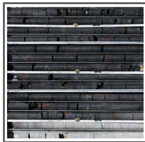
Photograph of core hole SES301RD prior to sampling for proximate analysis.
