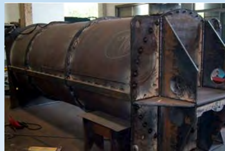
Sulphating mixer in fabrication
