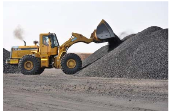
WCC's stockpiling of a -50mm thermal coal product to be sold to the domestic South African market
