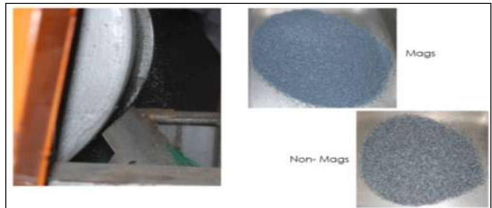
Coarse cobbing dry magnetic separation
