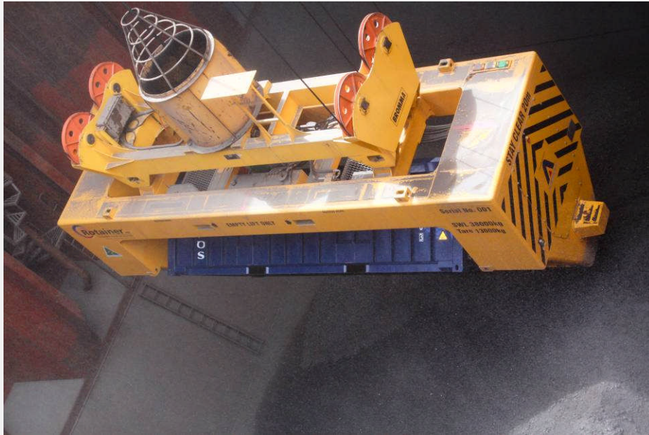
Figure 10: Container being rotated inside the hold of the vessel
