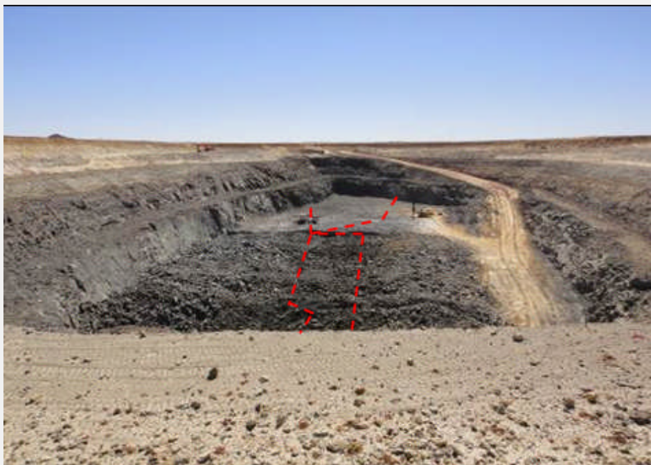
Figure 2: Starter Pit at end of December, looking east showing projected ore boundary on 110RL
