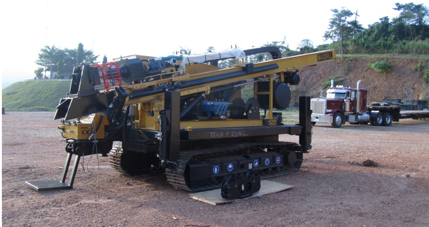
Figure 3 – Second Company owned multi-purpose drilling rig
