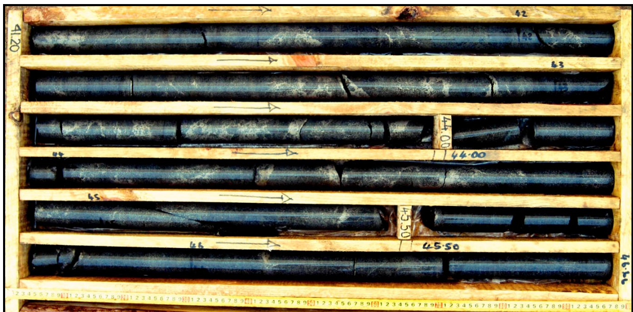
Massive and disseminated sulphides in Hole IPC0007 from 41.20m to 45.00m. The margins of this zone contain elevated chalcopyrite, with the bulk of the zone comprising pyrite / pyrrhotite.
