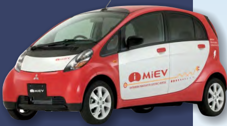
Mitsubishi MiEV is a full electric car powered by lithium ion batteries
