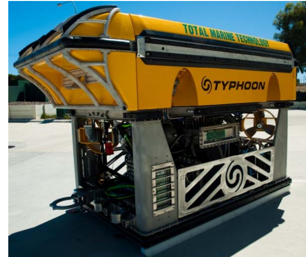
This ROV Utilises Matrix's Ultralight Carbon Fibre Syntactic Foam Buoyancy. **
