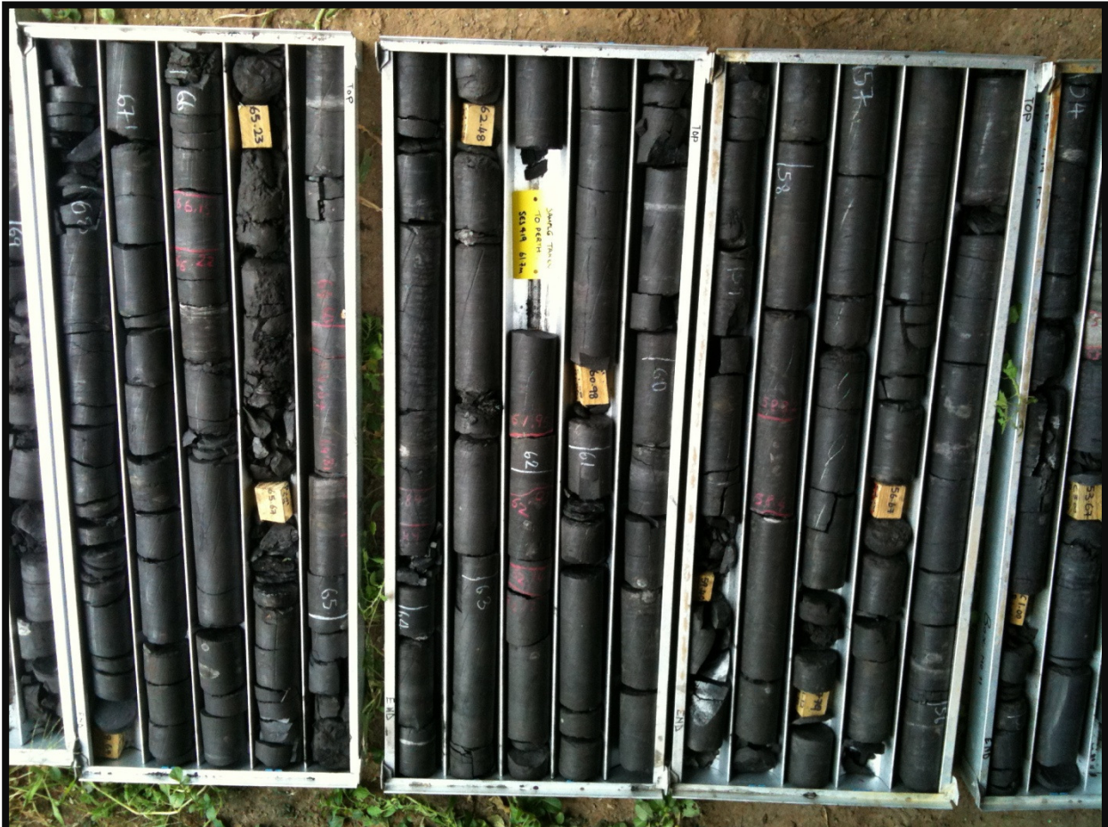
Picture 1: Intersection of coal in drill hole SES419 located in Block B of the Sese coal project. Photograph shows drill core from approximately 54m (top) to 69m (bottom) depth. Drill hole is oriented vertically.
