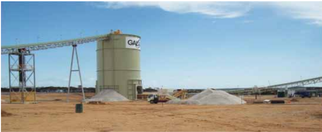
Figure 8.7 Crushed Ore Bin, with Recycled Product on Right
