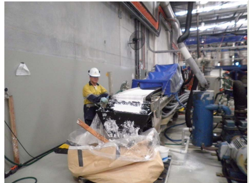
Gypsum production from Hydrochloric Acid regeneration demo plant at AMMTEC, Perth.
