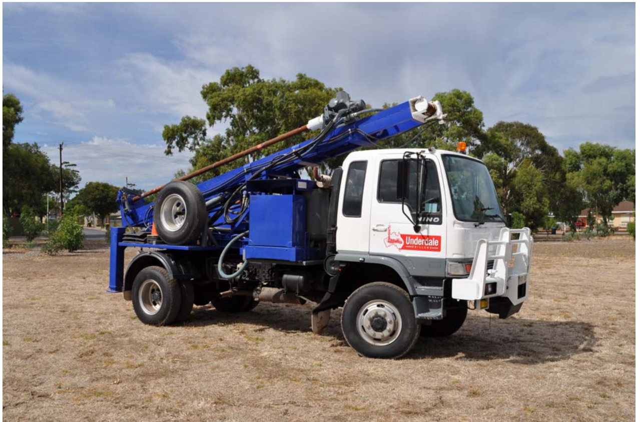
Figure 2: Underdale Drillers – Aircore Drilling Rig
