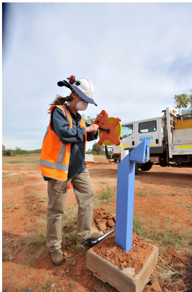
Water level monitoring as part of the Nolans Bore Mine EIS program.
