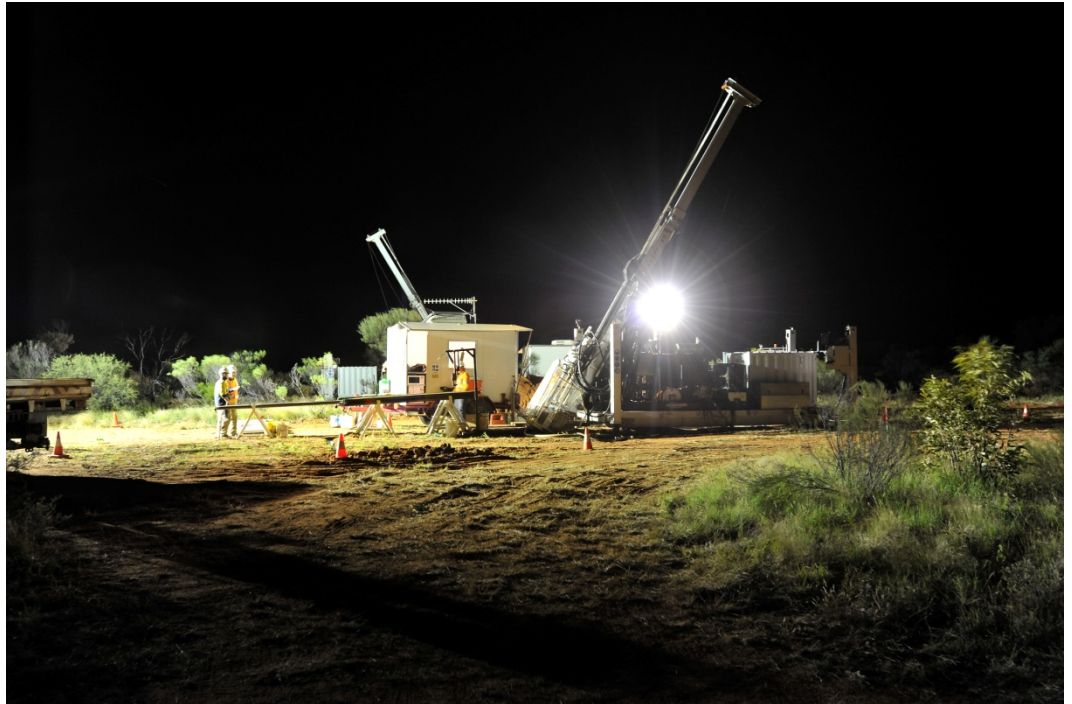
Night-shift diamond core drilling operations.
