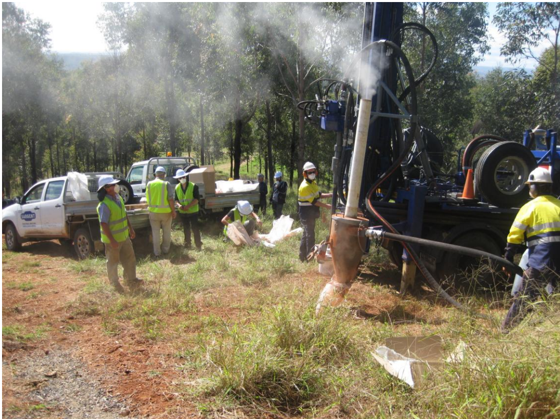
Figure 2: Kingaroy Project Monday 16 th May 2011 – Aircore Drilling Rig at work
