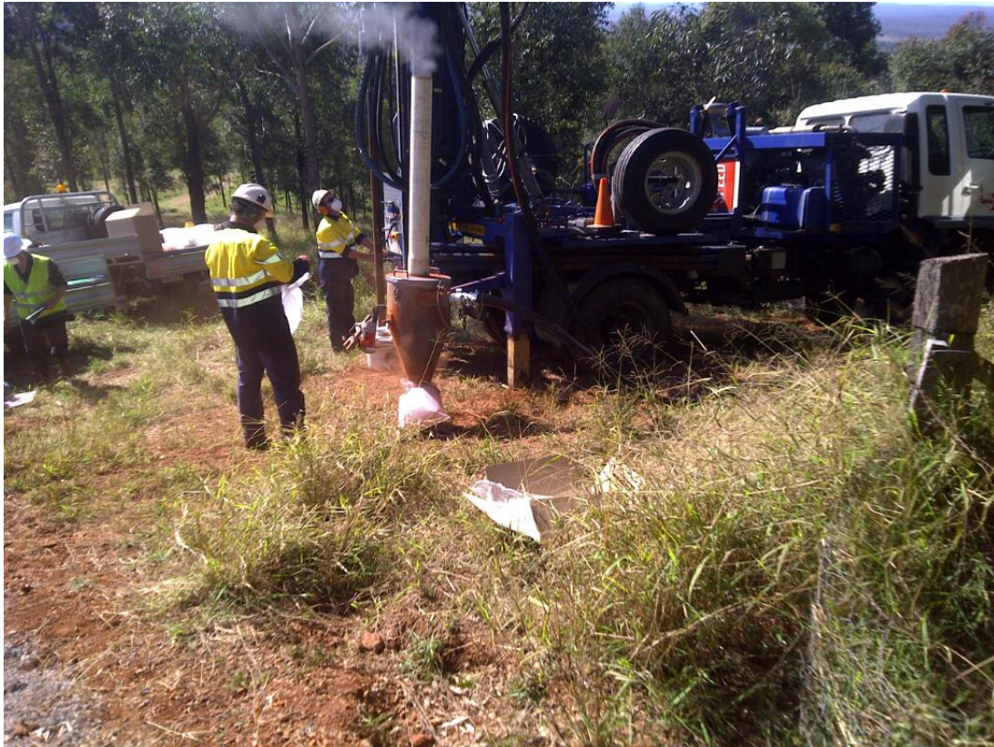
Figure 2: Kingaroy Project Monday 16 th May 2011 – Aircore Drilling Rig at work
