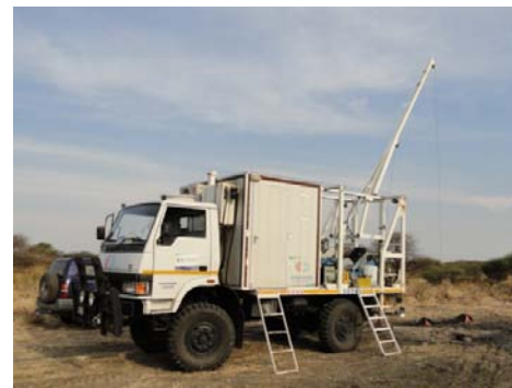
Down hole geophysical logging
