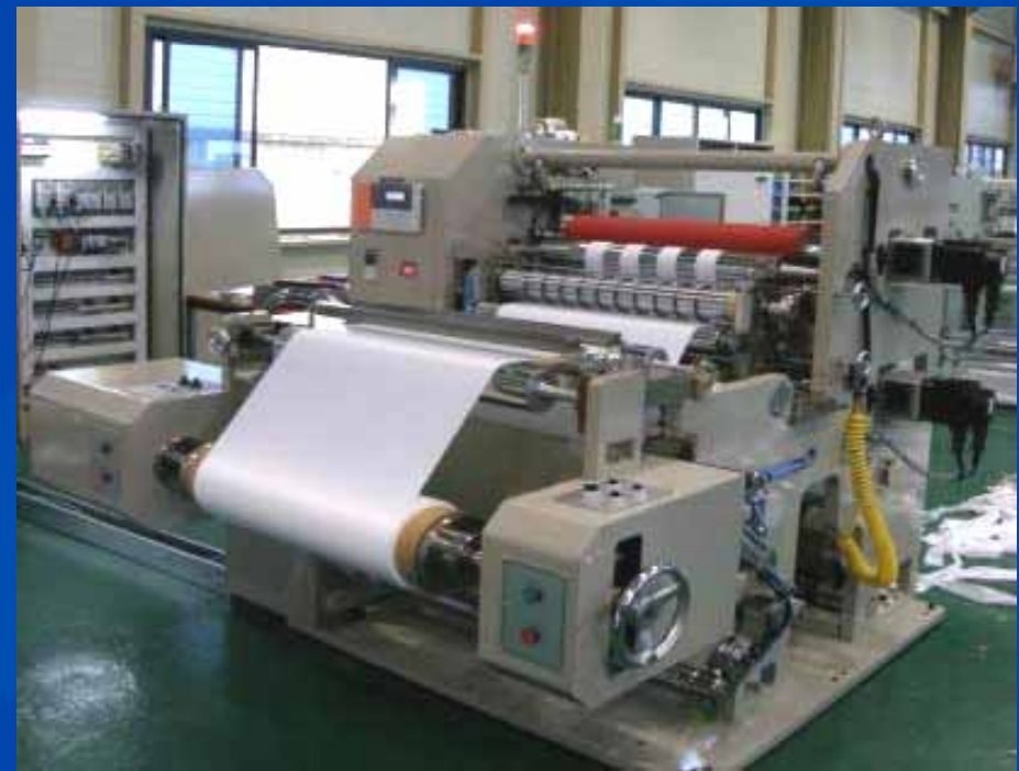
KUBT separator formation machinery
