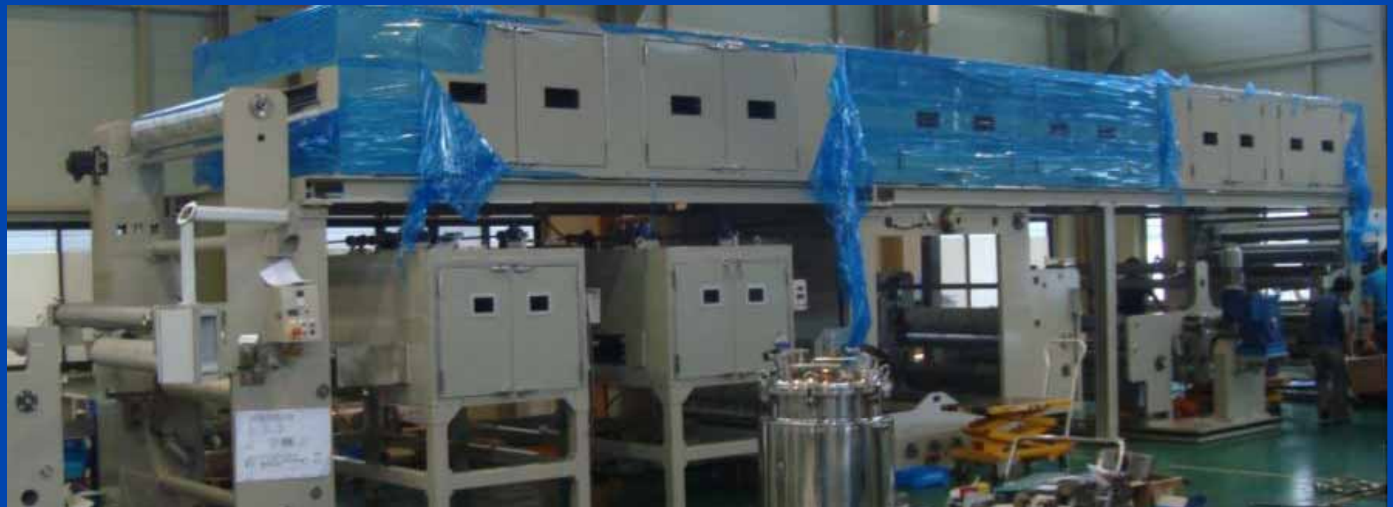
KUBT coating and drying machinery
