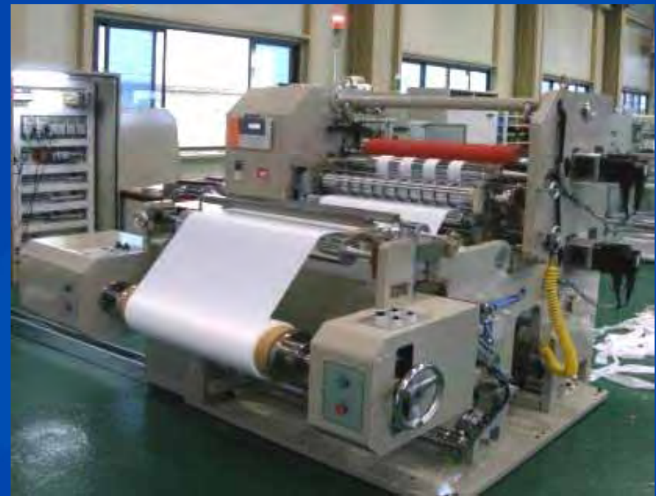
KUBT separator formation machinery
