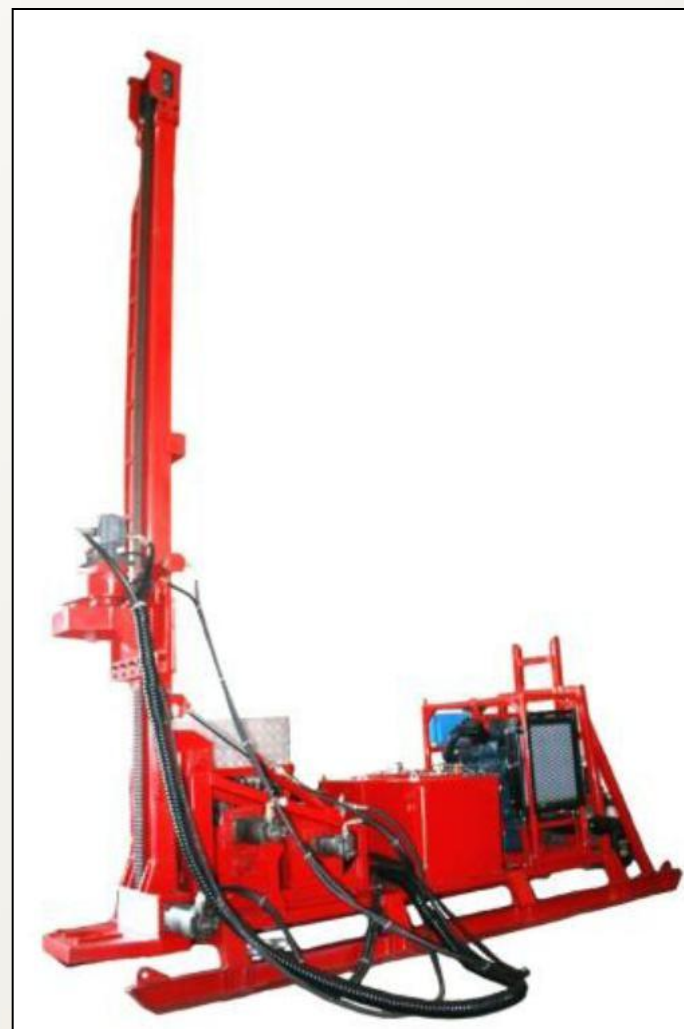
New diamond drilling rig built for Waratah
