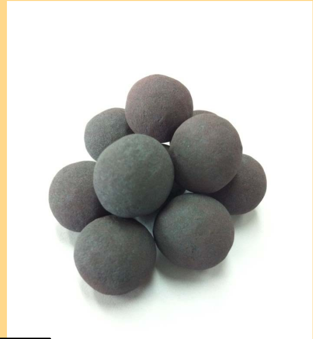
Pellets using local clay
