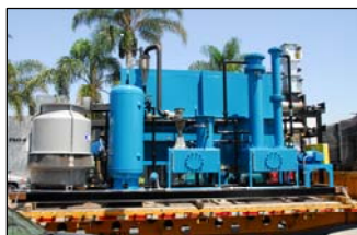
Municipal Waste Plant Gasifier
