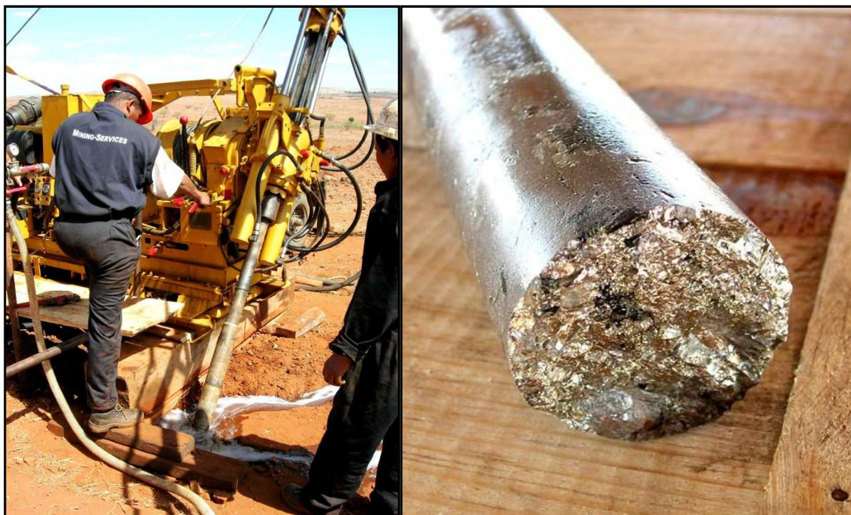
Left: Collaring the first hole (IPC001) at Ianapera Project. Right: Close-up of massive sulphides in IPC001.
