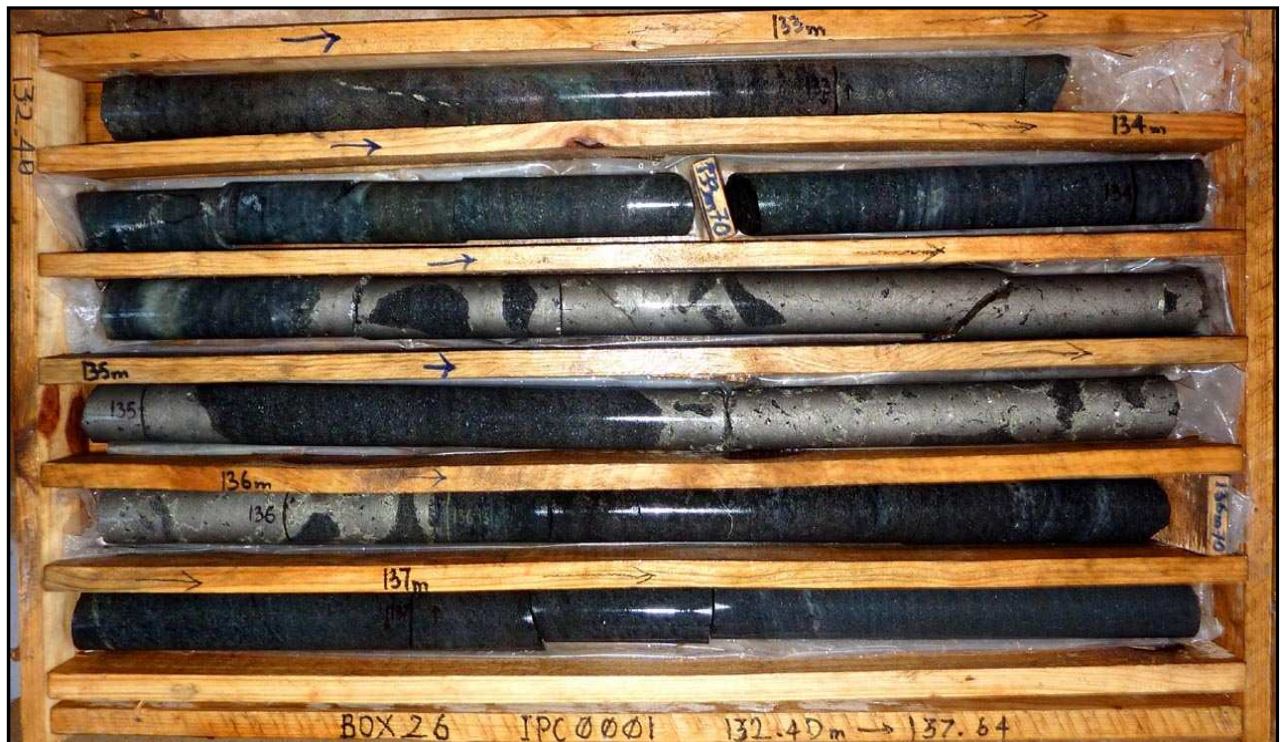
Massive sulphides in IPC0001 at the Ampanihy-Ianapera Project – an adjacent underlying 20m zone of disseminated (i.e. 5% to 15%) sulphides with chromite was also intersected – September 2010
