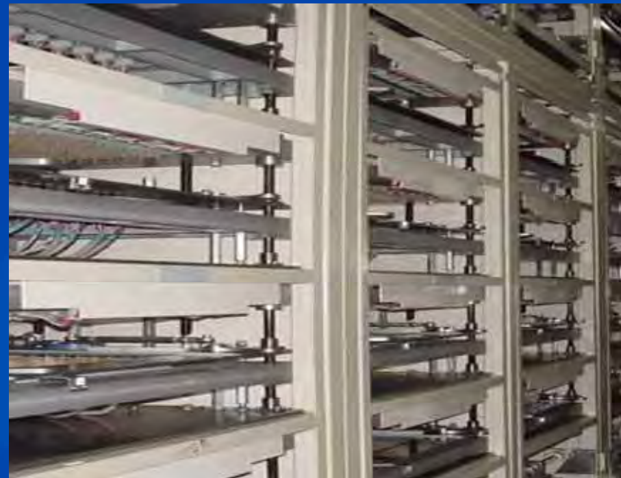
KUBT aging and degassing machinery
