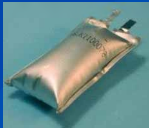
Gassing in prismatic cell
