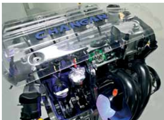
Changan's ICCS engine incorporating Orbital's FlexDI technology
