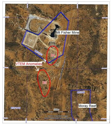
Figure 4: Mt Fisher Mine VTEM Anomalies, B4-B5
