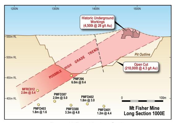
Figure 3: Mt Fisher Mine Long Section
