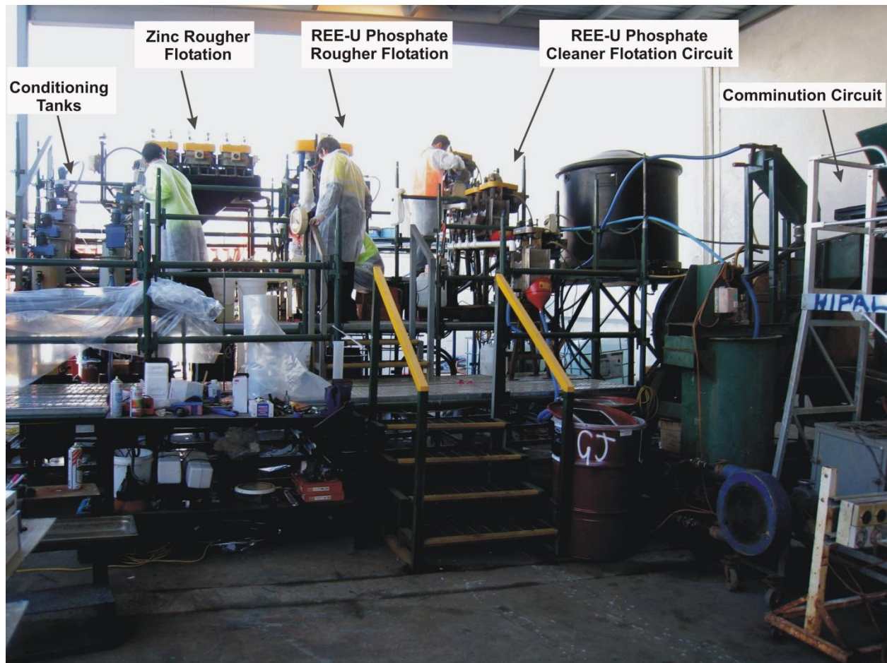
Figure 2. Kvanefjeld flotation circuit – stage one pilot plant, SGS Oretest, Perth. The plant was run continuously for 15 hours to produce a zinc (spalerite) concentrate, and a REE-U phosphate mineral concentrate. The ability to effectively concentrate the REE-U bearing phosphate minerals into a small mass fraction represents a critically important breakthrough in establishing the optimal process flow-sheet for the Kvanefjeld project.
