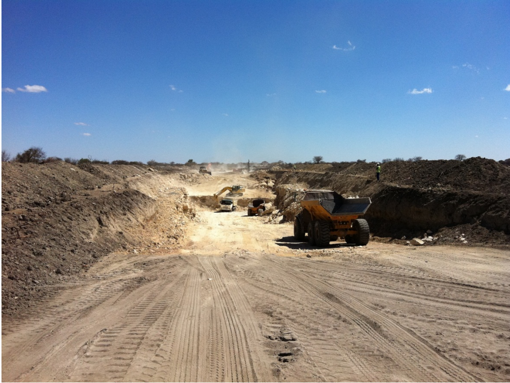
Diagram 5 Backhoe loading 20t and 40t trucks with blasted waste-material.
