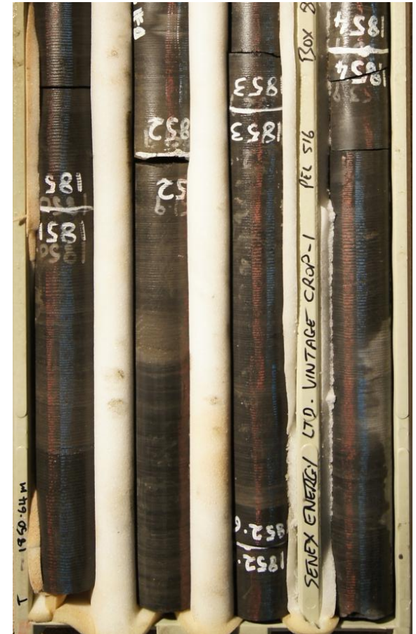
Vintage Crop-1 core samples - Roseneath Shale
