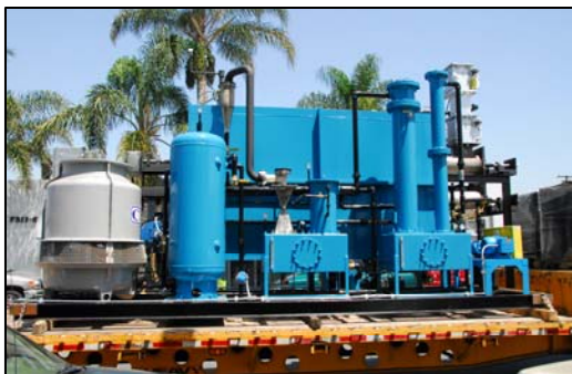
Municipal Waste Plant Gasifier
