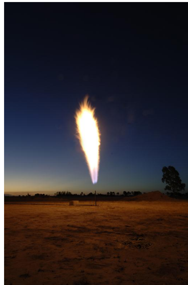
Coal seam gas appraisal well being flared
