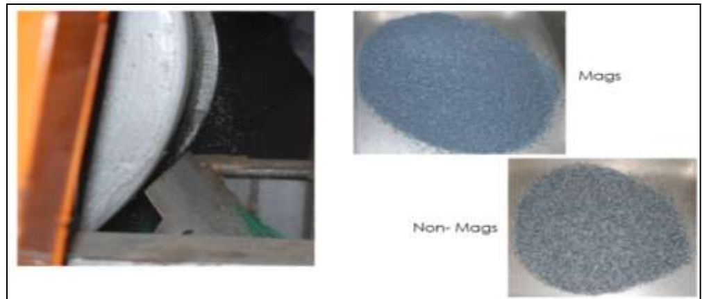
Coarse cobbing dry magnetic separation
