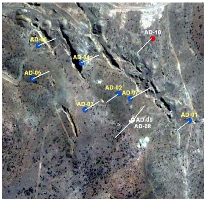
Blue dots show completed holes. Red dot shows current working hole.
