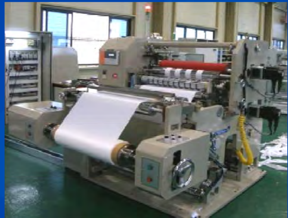
KUBT separator formation machinery
