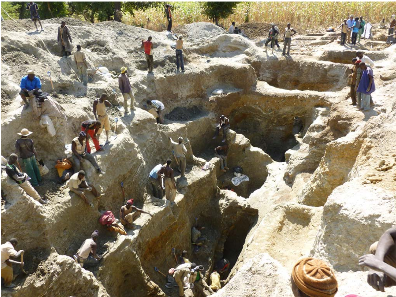
Figure 3: An example of the artisanal working present within Australian Mines' Kasele project area. Estimated depth of the working as shown in this figure is 10 metres. The quartz veining that hosts the gold mineralisation may be seen in this image as swarms of white layers within the walls of the working. As illustrated in this image, primary (or bedrock-hosted) gold mineralisation outcrops on surface across many parts of the Nigerian goldfields.
