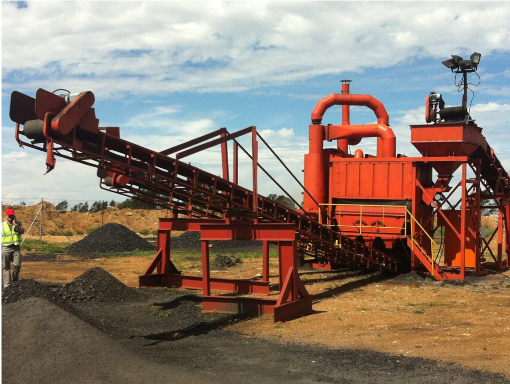
Diagram 8 10tph air separator pilot plant at processing facility in South Africa. This plant will be used for the first bulk processing trials of the initial 60t sample.
