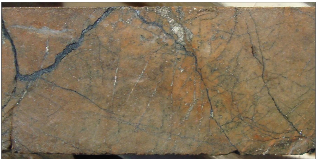
Metasomatite Rock: albite-chlorite-microcline rock with veins and fractures variously rich in quartz, carbonate, chlorite, pyrite
