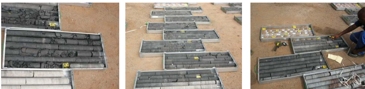
Diamond drill core from holes SRW02 and SRW04 to SRW05 on the Serowe Coal Project
