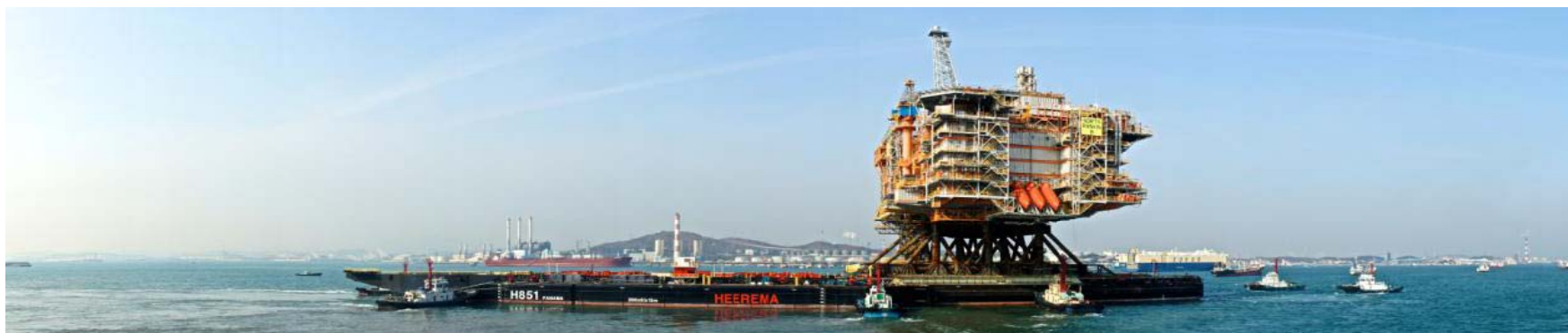
North Rankin B topsides unit on the heavy lift 'Heerema' barge, commences its journey from the Republic of Korea construction yards to the North West Shelf.
