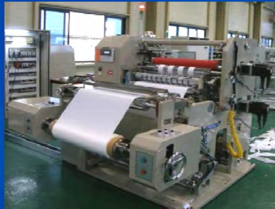
KUBT separator formation machinery
