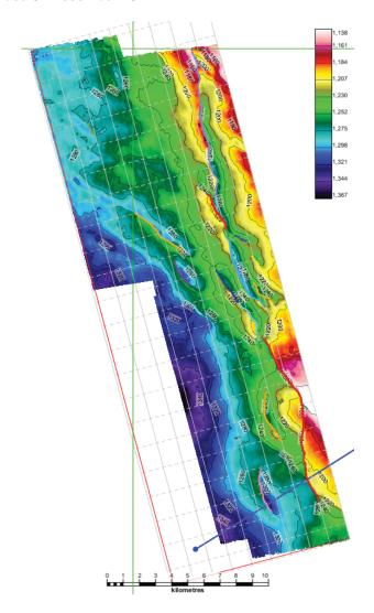
Preliminary mapping, of newly-processed Dalrymple 3D survey, of the top Eastern View Coal Measures (TWT).
