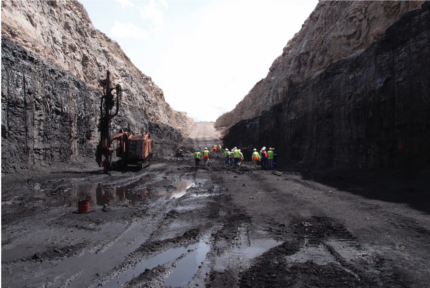
Sese bulk sample ramp. 15m of overburden above an 18m coal seam. Photograph depicts the upper 9m of the coal seam only.
