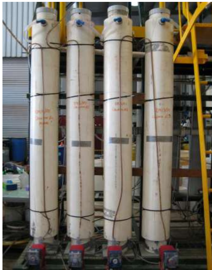
Figure 1: Häggån bacterial heap and tank leach testing at SGS Lakefield Oretest, Perth
