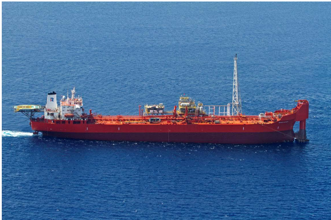
Figure 1: FPSO Rubicon Intrepid with bow mounted non-disconnectable turret installed
