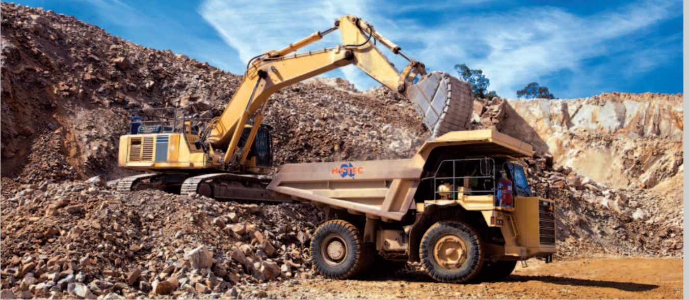
Top: Austen Quarry at Hartley, west of Sydney - loading of raw aggregate feed for processing in the crusher plant
